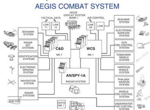
Gambar 4. Aegis Combat System Block Diagram.
